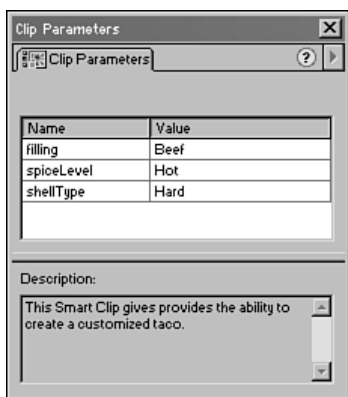
Figure 13.1 The author can specify variables uniquely for every instance of a Smart Clip by using the Clip Parameters panel.
