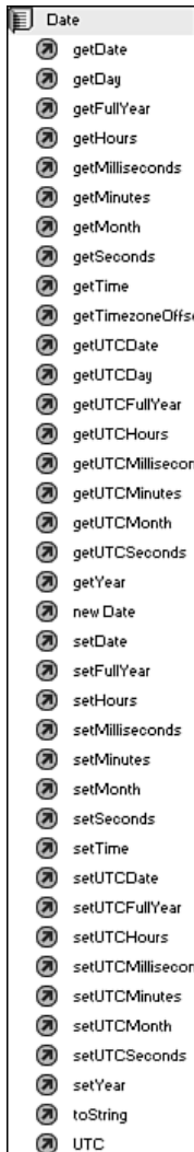
Figure 11.7 Although there are many methods for the Date object, they fall into two general categories—those that get values and those that set values.
